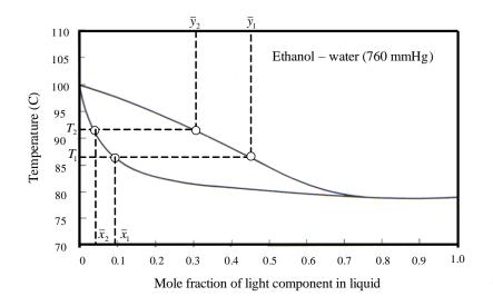
Figure 1. Vapor-liquid equilibrium of binary mixture at constant pressure.
