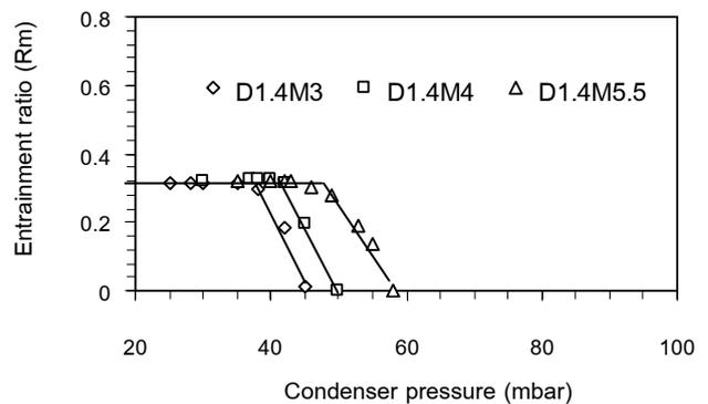
Fig. 6 Show the influences of nozzle's exit Mach number (by CFD simulation)
