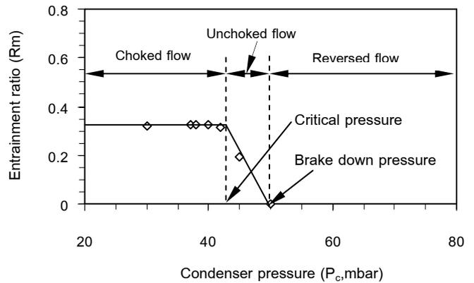
Fig. 3 The performance curve of steam ejector
