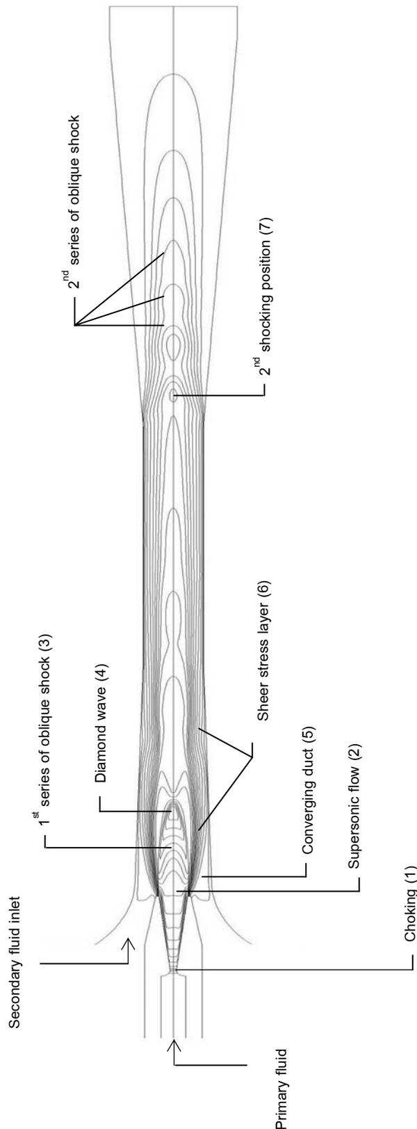
Fig. 2 Filled contour of mixing process within the steam ejector
