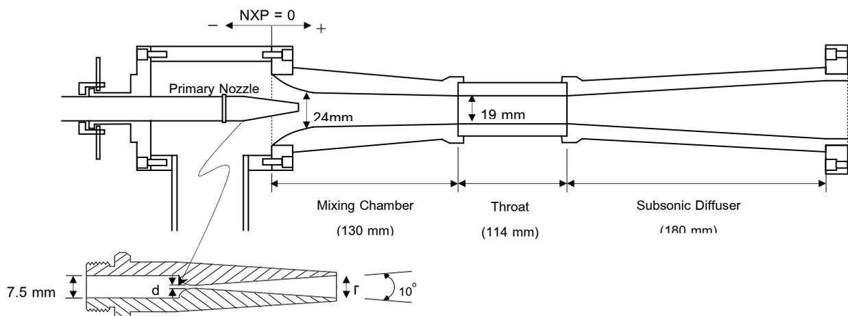
Fig. 1 Show the dimension of steam ejector used
