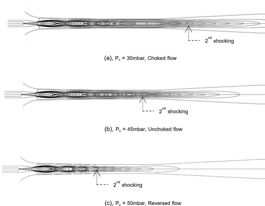
Fig. 4 the effect of condenser pressure ( $P_c$ ) on the 2<sup>nd</sup> shocking position
