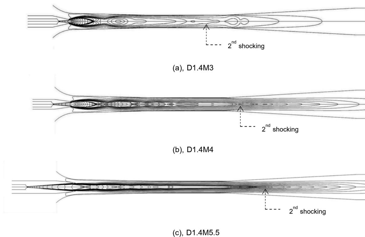
Fig. 7 The effect of nozzle's exit Mach number on the 2<sup>nd</sup> shocking position
