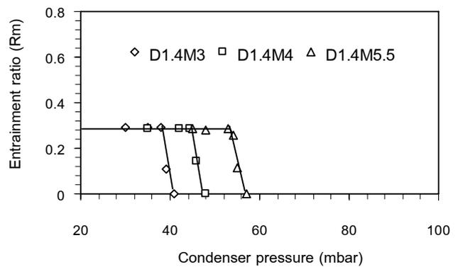
Fig. 5 Show the influences of nozzle's exit Mach number (by experiment)
