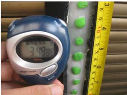
Fig. 2. Experimental apparatus for measuring infiltration front of water
