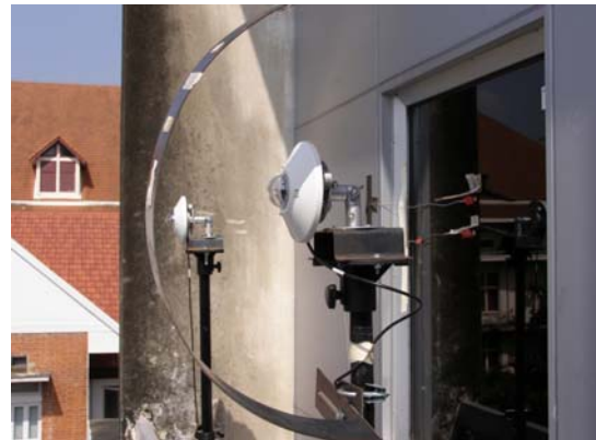
Fig. 7 Two pyranometers and a shading ring.
