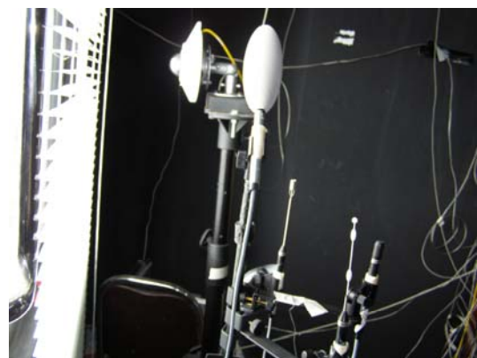
Fig. 8 Pyranometer used for measuring the transmitted solar radiation.
