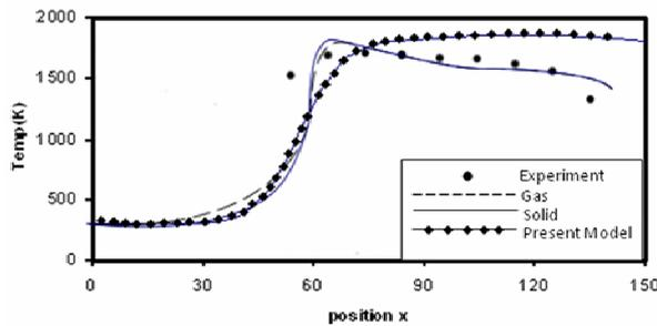
Fig. 3 Comparison of the centerline temperature from the present model, the previous model and experiment [8].
