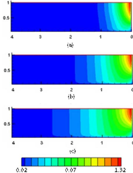
Fig. 6 Distribution of  $u$ -component velocity at different time,  $\bar{t}$  of (a) 0.5, (b) 1.5 and (c) 3.0.
