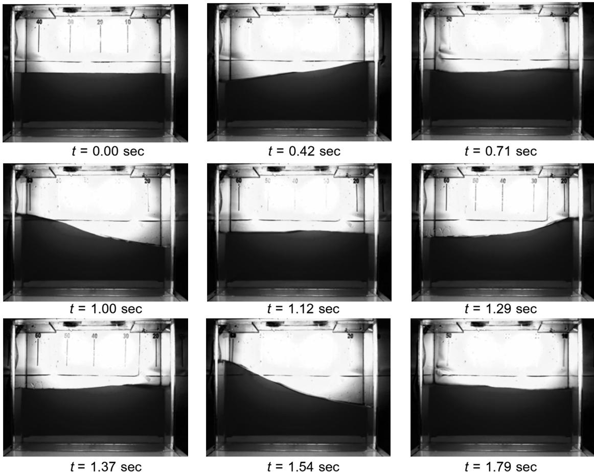
Fig. 4 Sequential gray images of the surface wave using Grayscale toolbar in the SloshDetector software.
