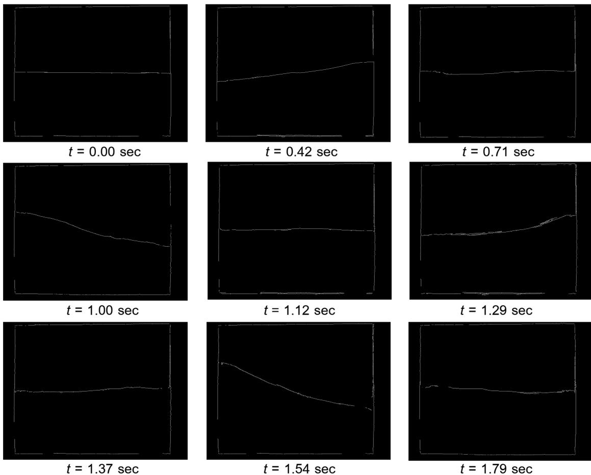
Fig. 6 Sequential images of detected surface wave using the Canny toolbar in the SloshtDetector.
