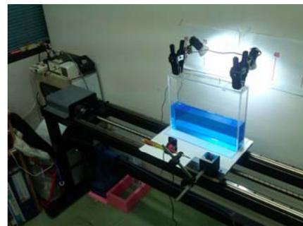
Fig. 1 Apparatus of experimental device for sloshing.
