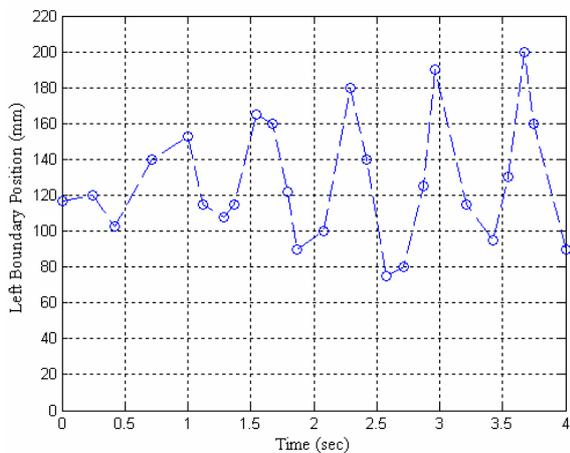
Fig. 10 The height of the surface wave at the left wall of tank vs. time.
