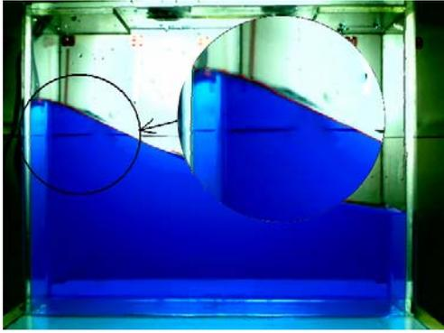
Fig. 7 The detected surface wave overlapping on the original image at  $t = 1.54$  sec.
