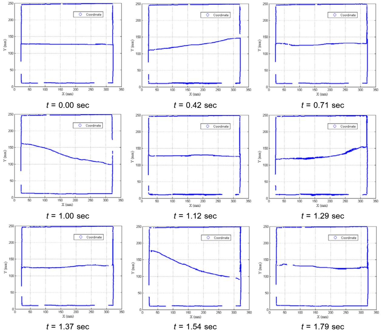
Fig. 9 The sequential plots of the surface wave for time = 0.00 sec to time = 1.79 sec using the SlosHDetector software.
