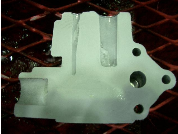
Fig.7 Color-check testing result (As-Cast)
