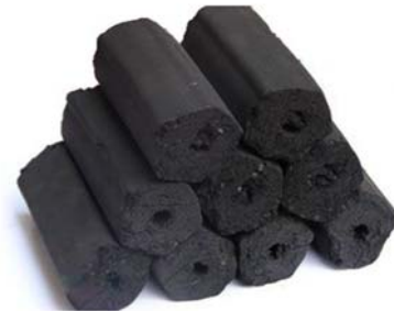
Fig. 7 Briquettes obtained from the compact machine
