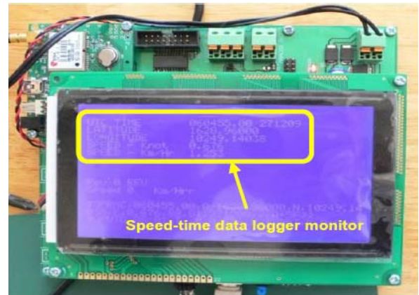
Fig. 1 Monitor of the data logger system
