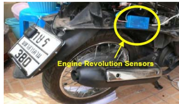
Fig.4 The signal receiving unit from the Capacitor Discharge Ignition (CDI)
