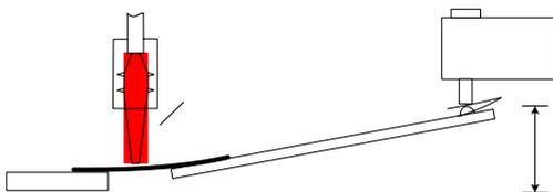
Fig. 2 Heat treatment by laser process
