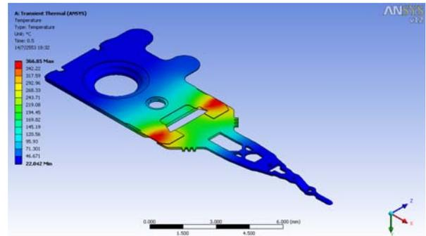
Fig. 6 - 1 The temperature distribution on hinge.
