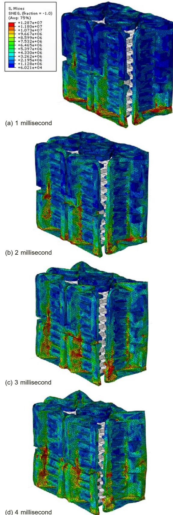
Fig. 7 Stress distribution on the cushions at 1 to 4 milliseconds of seq 7
