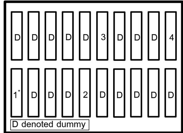
Fig. 2 Positions of hard disk drives (1-4) and dummies (D)
