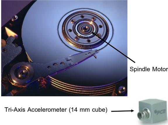
Fig. 3 Tri-axis accelerometer installed at spindle motor
