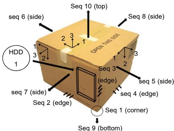
Fig. 4 Sequences and local directions of drop test (First hard disk drive shown)
