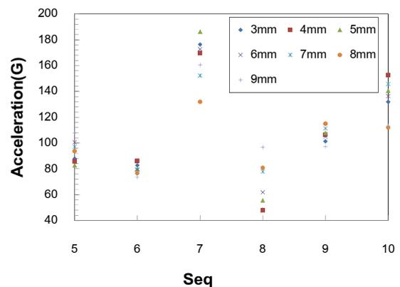
Fig. 6 Acceleration on HDD position 1 for various cushion spacing ( $d$ )
