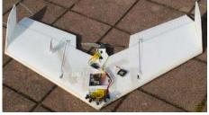
Vision based MAV of LIS-EPFL, span 80cm
