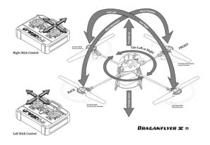
Fig. 8 The control methodology of Quadrotor
