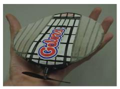
Gators MAV, The University of Florida Fig. 5 Flexible Wing Based MAV, FL
