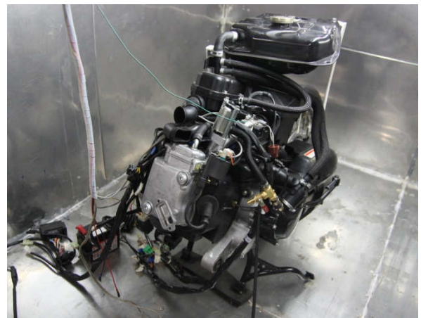
Fig. 3 Suzuki Skydrive engine in the cold soak chamber
