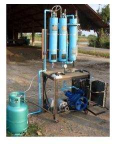
Figure 5 Biogas Compression Systems
