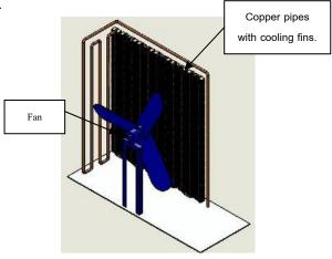
Figure 4 Biogas cooling System
