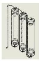
Figure 3 Biogas Scrubbing System
