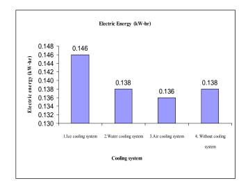
Figure 8 Comparison of electric energy consumption
