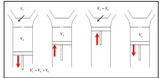
Figure 1 Operation of the piston
