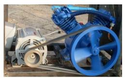
Figure 2 Biogas compressor and motor
