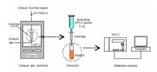
Fig. 2 schematic diagram of exhaust gas sampling for aldehyde analysis
