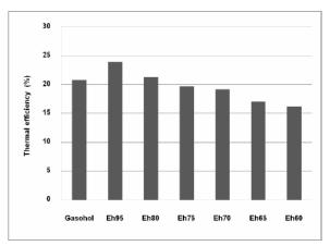
Fig. 4 Thermal efficiency with various water contents in ethanol at 3300 rpm, 4 kW load and stoichiometric A/F ( $\lambda$ =1).
