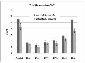
Fig. 8. Total hydrocarbon from combustion of hydrous ethanol with various water contents at 3300 rpm, load 4 kW and stoichiometric A/F.
