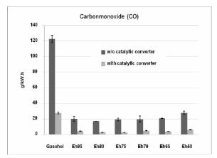
Fig. 7. Carbonmonoxide from combustion of hydrous ethanol with various water contents at 3300 rpm, load 4 kW and stoichiometric A/F.
