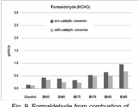
Fig. 9. Formaldehyde from combustion of hydrous ethanol with various water contents at 3300 rpm, load 4 kW and stoichiometric A/F.
