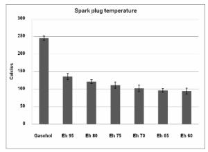
Fig. 6. Spark plug temperature at 3300 rpm, load 4 kW and stoichiometric A/F.
