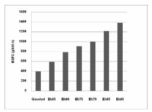
Fig. 3. Brake specific fuel consumption with various water contents in ethanol at 3300 rpm, 4 kW load and stoichiometric A/F (λ=1).
