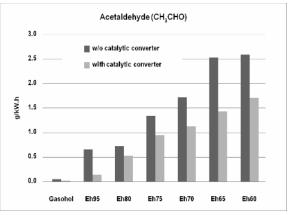
Fig. 10. Acetaldehyde from combustion of hydrous ethanol with various water contents at 3300 rpm, load 4 kW and stoichiometric A/F.
