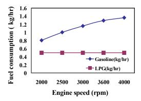
Fig. 7 Fuel consumption of gasoline and LPG at different engine speed
