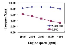
Fig. 5 Relationship of output torque at different
